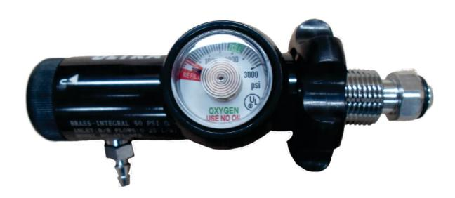
Dial Click Stop Constant Flow with pressure gauge to register cylinder pressure Oxygen delivery through Click-Stop Hand Dial Marked 0-25I/min Oxygen Cylinder Pressure Gauge Pressure Dial protected by a rubber ring Outer Body manufactured from Aluminium **Inner Body Manufactured from Brass** Minimum Input Operating Pressure 200 bars Output Pressure at Heyer: 3 - 6 Bar **Complete Male/Female Connection Included**
