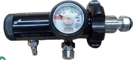
Dial Click Stop Constant Flow with pressure gauge to register cylinder pressure Oxygen delivery through Click-Stop Hand Dial Marked 0-25I/min Oxygen Cylinder Pressure Gauge Pressure Dial protected by a rubber ring **Outer Body manufactured from Aluminium Inner Body Manufactured from Brass** Minimum Input Operating Pressure 250 bars
